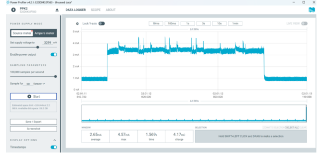
Fig. 5. Experimental platform based on NRF52840 Development Kit and PPK II and square wave current diagram on laptop
